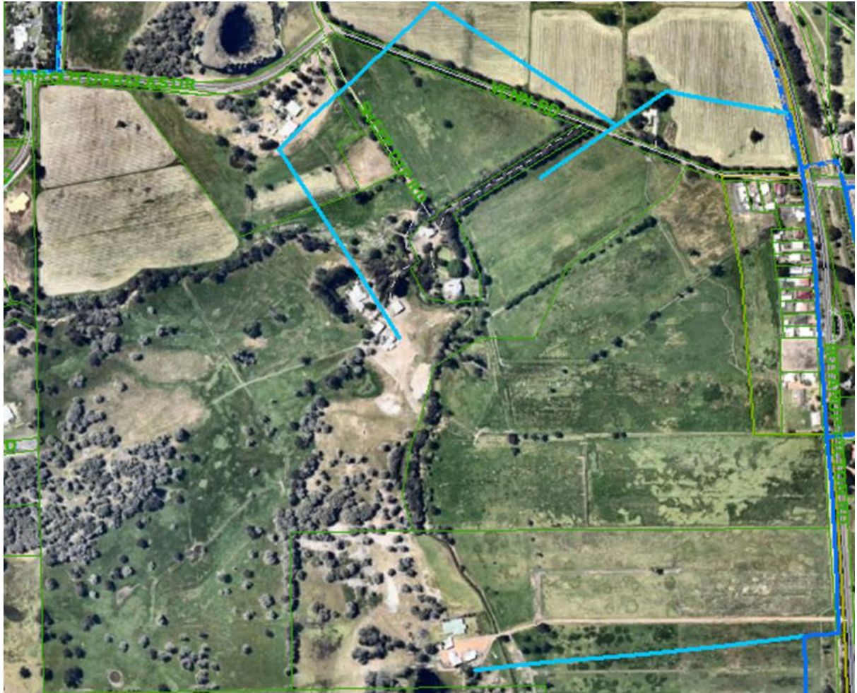
Figure 4: Present HV Network Dark blue is three phase. Light blue is single phase.
